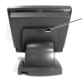
Press the Lock/Release button and lift the main unit to detach it from the stand assembly.
